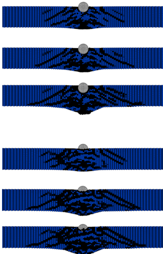
Figure 8: (a) Numerical by NSNI and experimental [13] cracking patterns; Top: cross sections of the cracking pattern at the point of impact, Bottom: cross sections of the cracking pattern away from impact; (b) Top: lateral cracking in numerical simulations, Bottom: lateral cracking in a brittle impact experiment [14].
